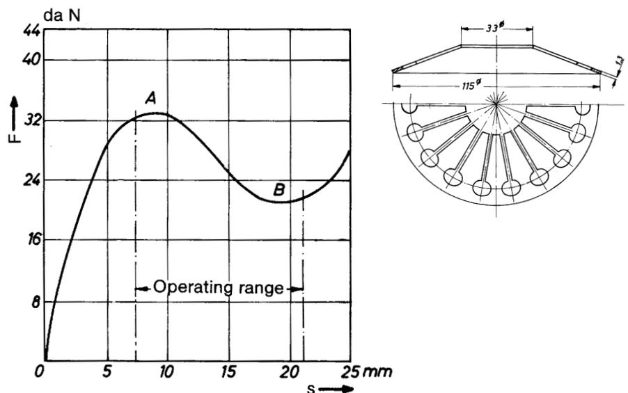
Fig. 18: HAUSSERMANN Diaphragm Spring with partly negative characteristic for use in V-belt transmission for stepless speed control
