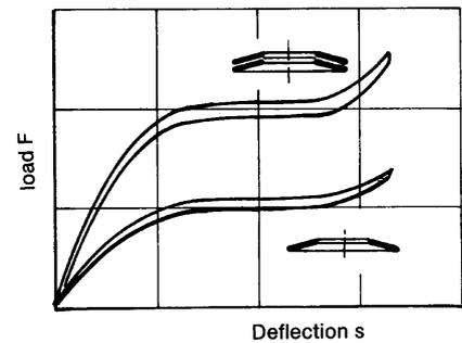
Fig. 11: Increasing the spring force by parallel stacking
