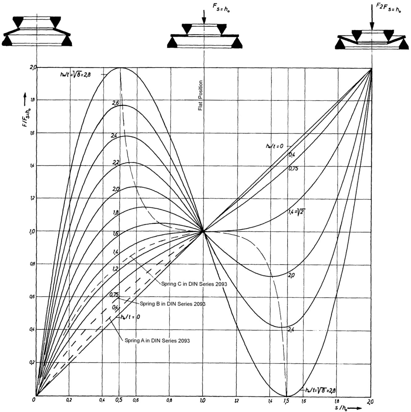
Fig. 5: Family of characteristics of the Diaphragm Spring, with variable  $h_0/t$
