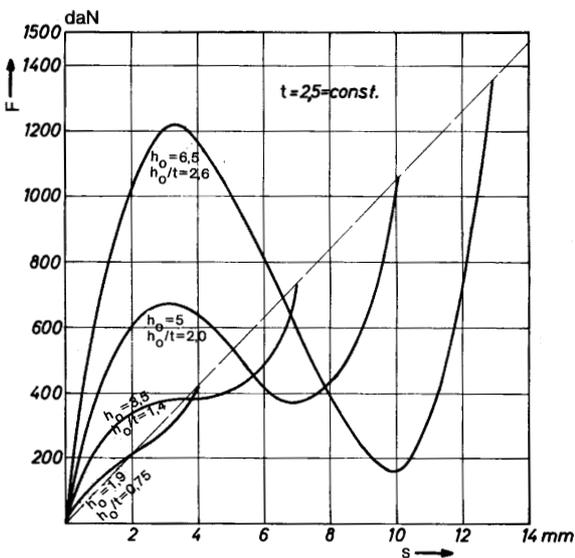
Fig. 3: Outline of characteristic as a function of  $h_0/t$ , where  $t = \text{constant}$
