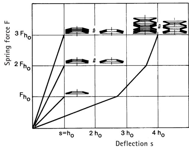
Fig. 7: Spring combinations with progressive characteristics (diagrammatic, disregarding friction)
