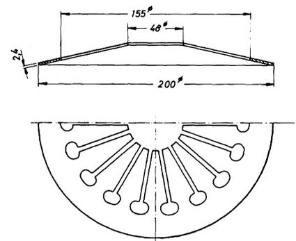
opening width is set, and the opening of the secondary pulley is adjusted automatically. Slotted diaphragm type springs provide the pressure required for the adhesion of V-belts. The large deflection range necessary for the ultimate variator setting is obtained by means of a diaphragm spring having extended fingers and a large conical height.
