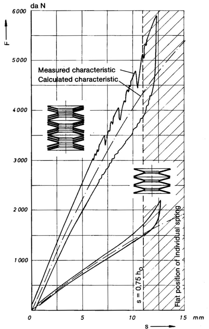
Fig. 9: Influence of friction (damping) upon the spring characteristics of two sets of parallel and series stacked spring combinations. (Springs B 90 DIN Series 2093)
