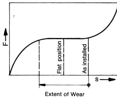
Clutches so equipped require no readjustment other than renewal of friction elements, and thus are free of maintenance. Frequently disc springs with an  $h_0/t$  ratio of 1.3 are used in these cases. However, these springs do not actually have a horizontal portion and have to be stacked to give the required deflection. Therefore, as wear takes place, the load reduces with an increasing tendency for the clutch to slip.
