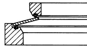
*Pivot rings inserted in groove.*
