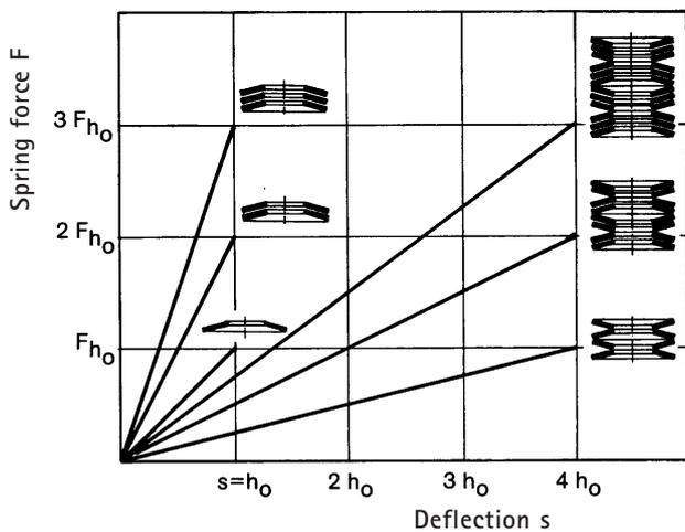
Fig. 6: Characteristics of different spring combinations (diagrammatic, disregarding friction)
