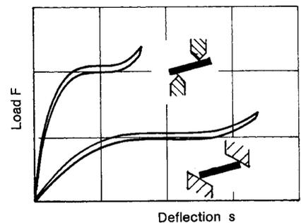
Fig. 12: How a reduction of support leverage affects the spring characteristic.
