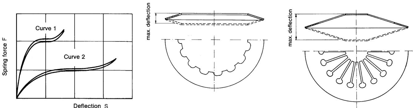
Fig. 13: How an extension of support leverage affects the spring characteristics
