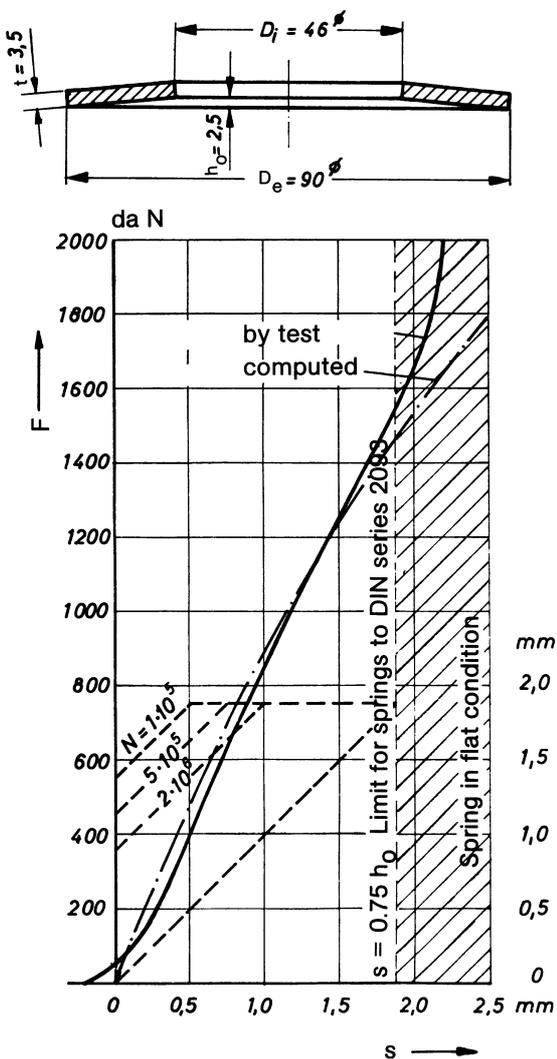
Fig. 8: Dimensions and spring characteristic of a B 90 DIN 2093 Standard disc spring
