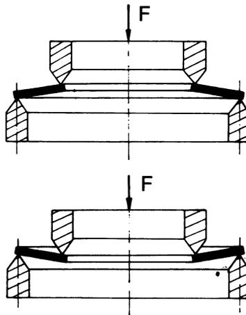
Fig. 10: Function of a diaphragm spring with extended deflection range.
