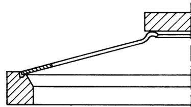
*With a flat compression piece, the finger tips will be cranked and hardened.*
