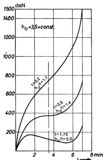
Fig. 4: Outline of characteristic as a function of  $h_0/t$ , where  $h_0 = \text{constant}$
