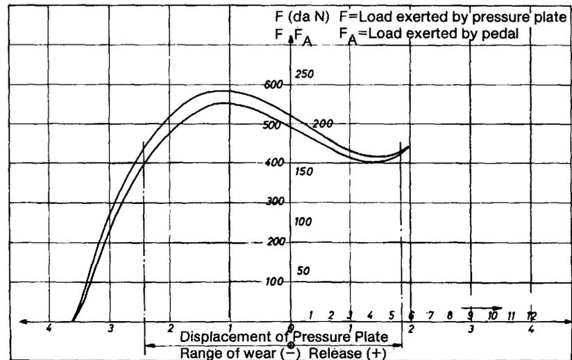
Fig. 17: HAUSSERMANN Diaphragm Spring with partly negative characteristic for use in passenger car clutches. Spring characteristic and section of clutch (diagrammatic)
