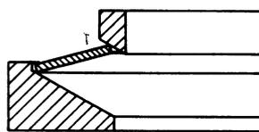
*Diaphragm spring between inclined planes. In cases of high dynamic loading, it is recommended that the support edges of the spring be rounded off.*
